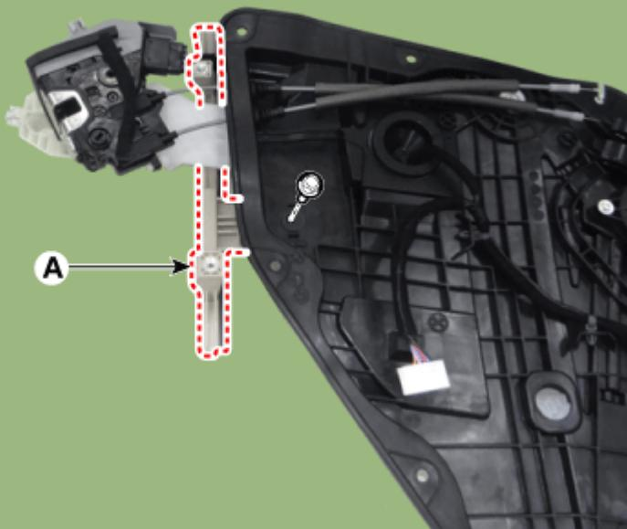
10. Remove the rear door latch (B) after disconnecting the latch connector (A).
